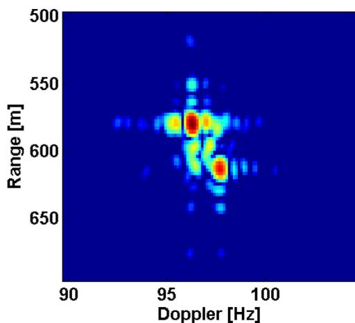
**Figure 7.** ISAR image using SAP of an Airbus 321
