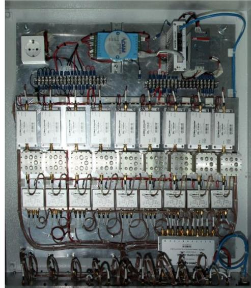
Figure 5. Antenna array (designed by ENAL) measurements in anechoic chamber (left) and calibration network (right)
