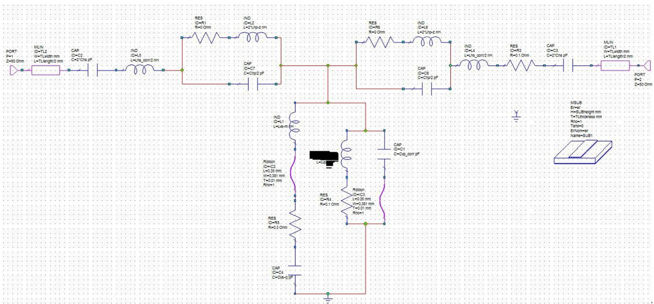
This unit cell has its host Transmission Line length included in it and its effects are taken into account in the calculation of the required component values. The figures below show the magnitude and phase data of these unit cells
