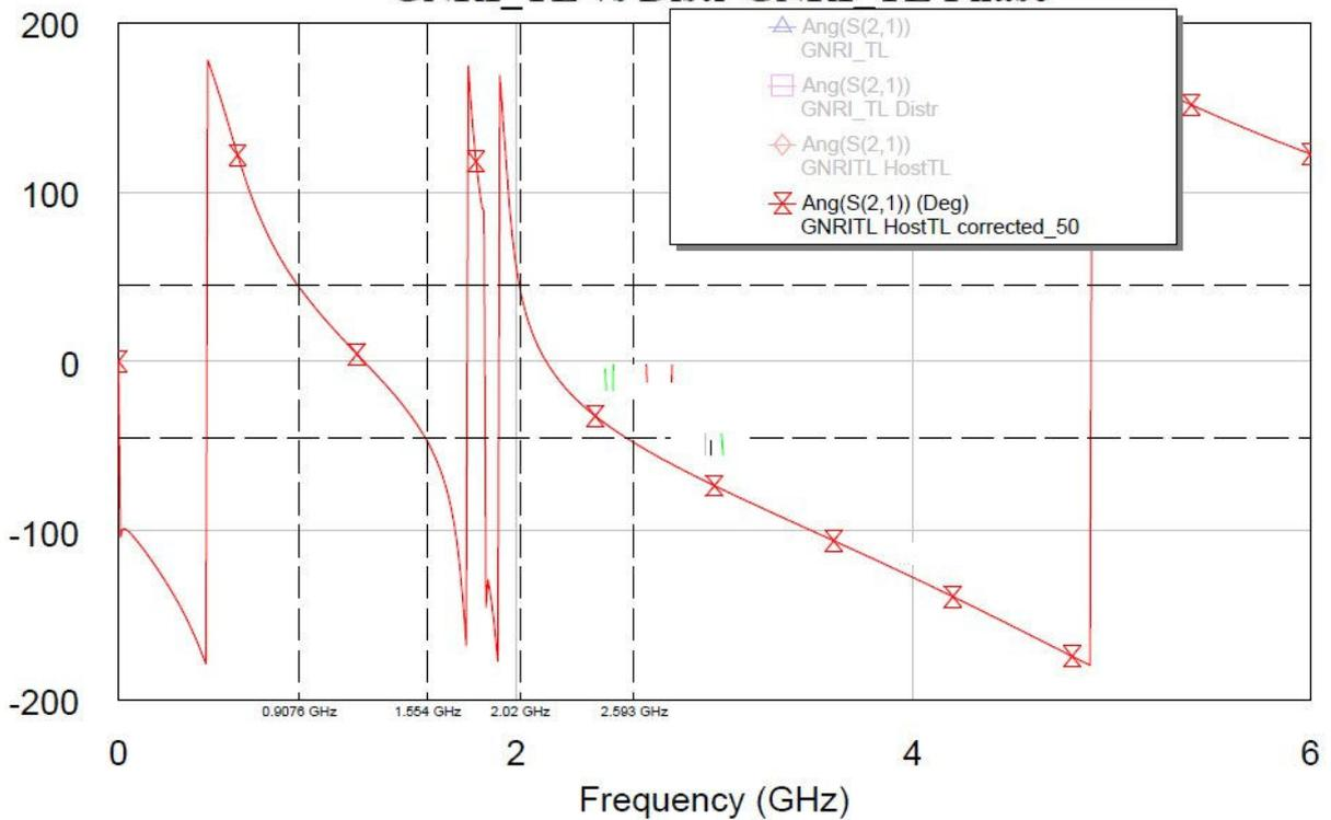
The next step in the design process was to design the unit cells in the full-Wave EM simulator to verify the magnitude and phase performance. This is the final step before the generation of the gerber layout files that are used for the board fabrication of the unit cells.
