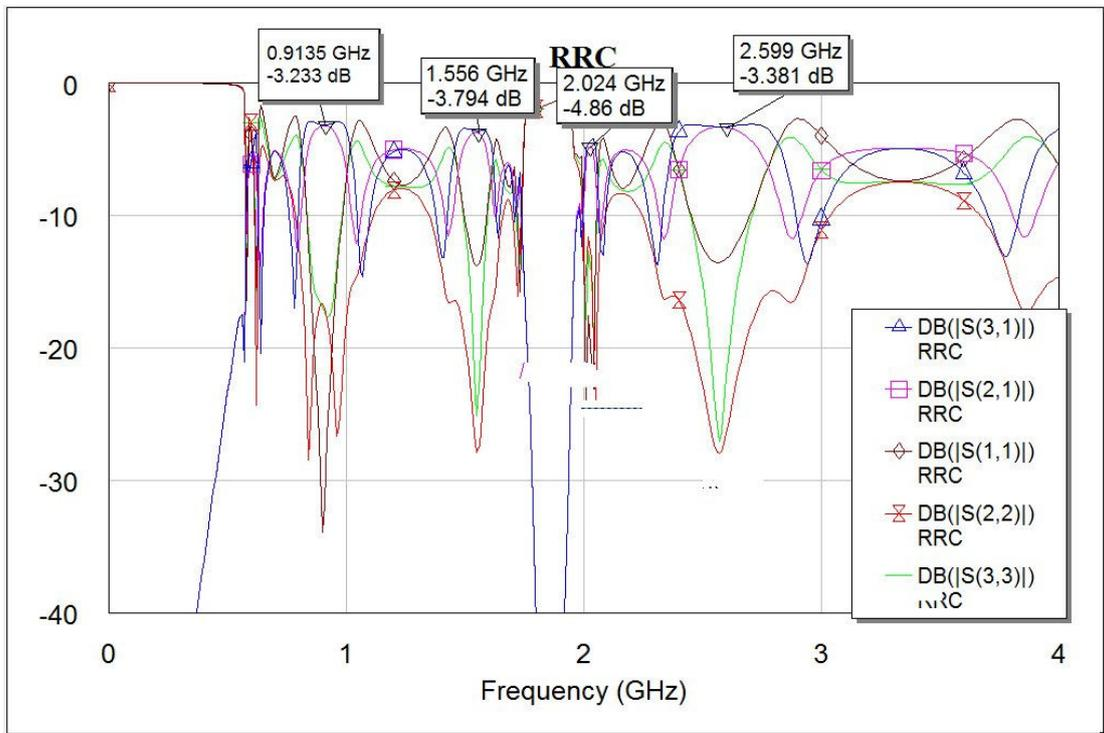
From the above graph, it can be seen that the insertion loss at the four design frequencies is acceptable and thus validation of the rat-race coupler concept using NRT-TL unit cells is complete.
